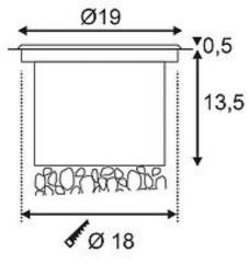
Walkable, low-voltage recessed ground luminaire with round stainless steel cover and partially frosted glass. Rated IP67, it it suitable for outdoor use. To ensure accurate illumination, the lamp is adjustable. The electrical connection is made directly to 230V mains supply via the incorporated transformer. For simplified mounting, a installation housing is included. This luminaire is compatible with bulbs of the energy classes: D - A+
